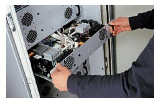
**Replaceable.** The individual printed circuit boards – up to 15 – are easy to pull out because of the plug-in racks. They also enable optimum utilisation of the inverter and therefore maximum output.
