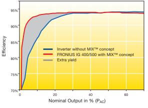
**Increase in output.** The MIX<sup>™</sup> concept converts part-load into fullload. Therefore, efficiency is increased and the yields are optimised in the part-load area.
