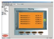
**FRONIUS String Control.** The optional single string monitoring system allows 25 strings to be monitored separately per box with up to 5.000 strings in the overall system. This means more security for reliable energy production.
